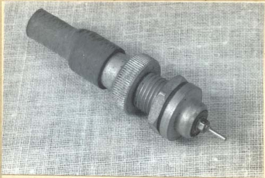
PYE MIN. CO-AXIAL SEALED PLUG & SOCKET
