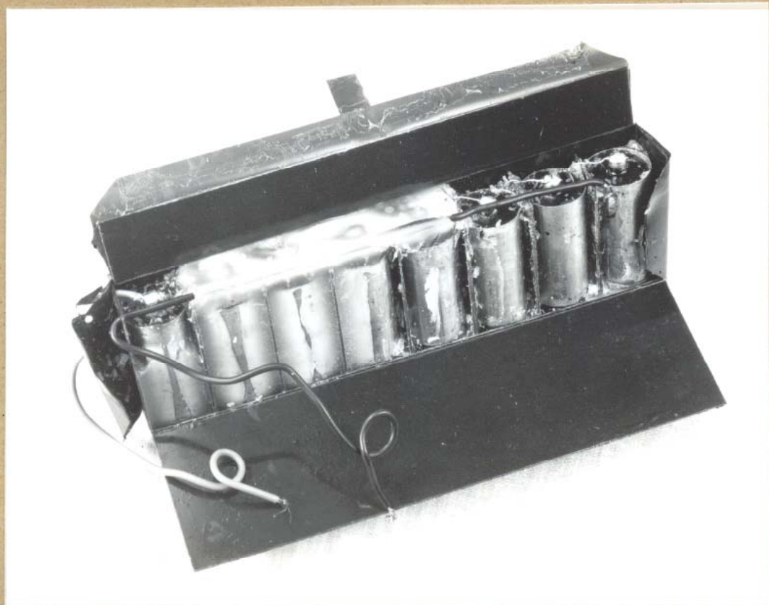
12-VOLT BLOCK, EXPLODED
